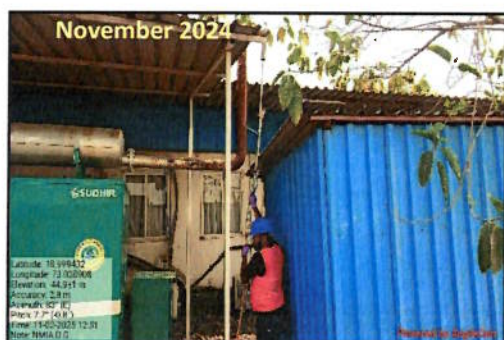
Figure 4-17 DG Stack Sampling
