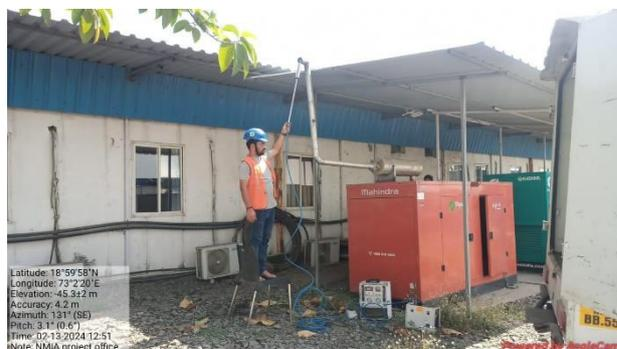
**Figure 4-17 DG Stack Sampling**
